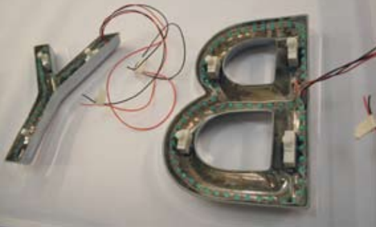
Fitted with LED'S for a halo effect
